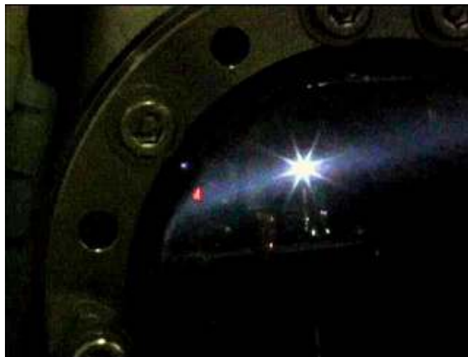
Figure 9 Picture of magnetic field guided LPP plasma
