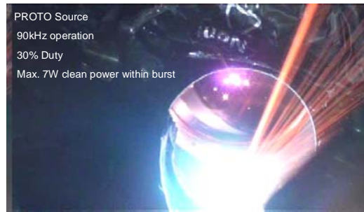
Fig.18 Picture of proto EUV source operation (2011)
