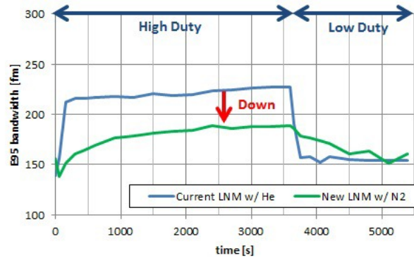
Fig.6 Results of heat effect without bandwidth control in new type LNM The heat effect in new type LNM with Nitrogen gas is smaller than that in current type LNM with Helium gas.
