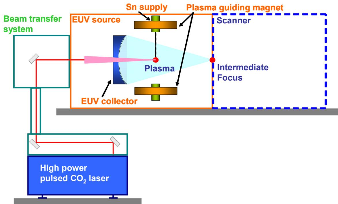
Figure 1. LPP EUV light source System
