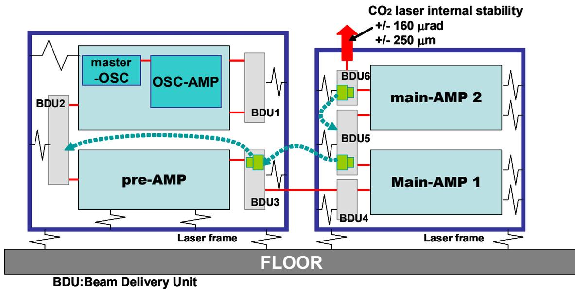
Figure 2. CO<sub>2</sub> laser system configuration
