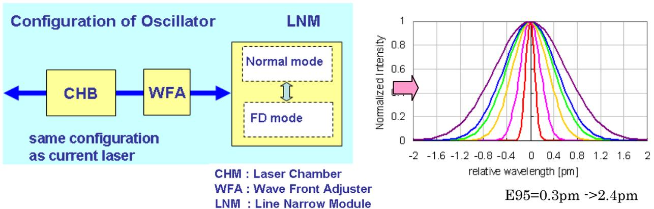
Fig.4: How spectrum bandwidth tuned
