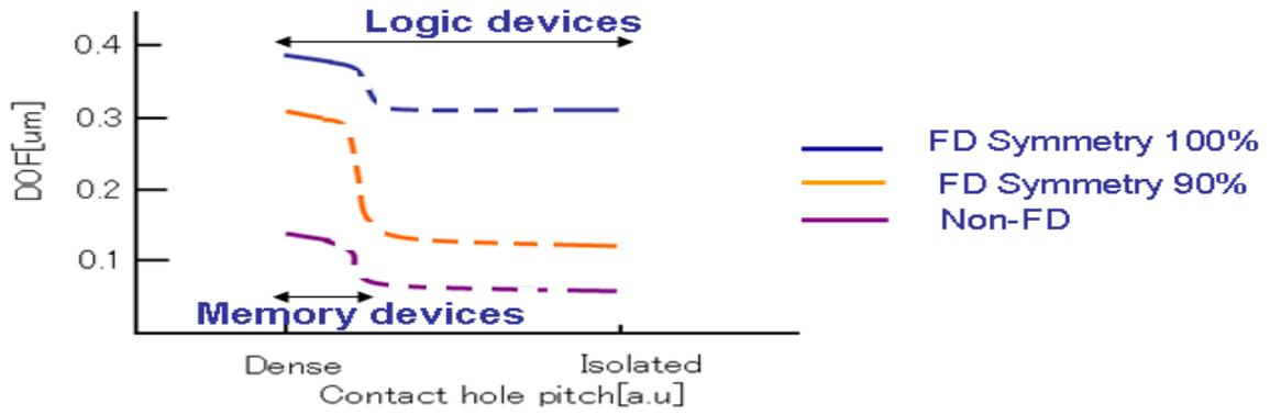
Fig.1: Relation between contact hole pitch and DOF
