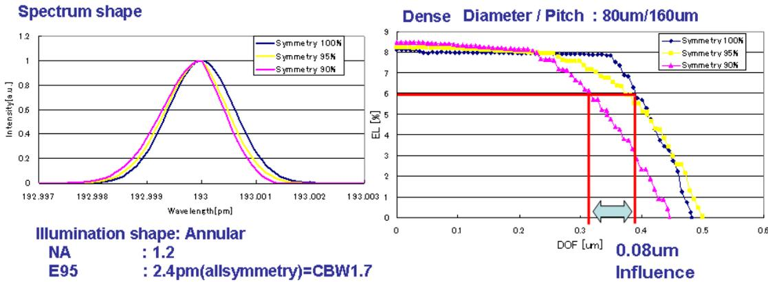
Fig.5: Correlation of the symmetry of spectral shape and DOF (Dense)
