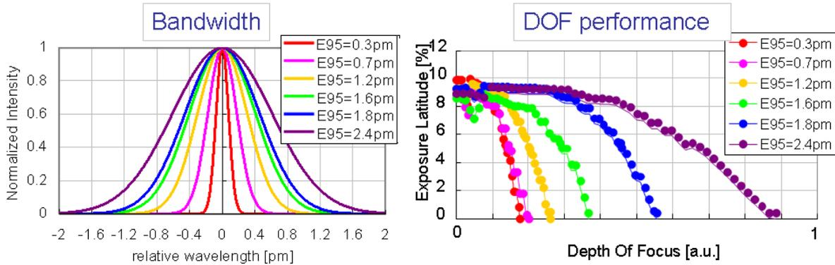
Fig.3: Correlation of spectral band width and DoF
