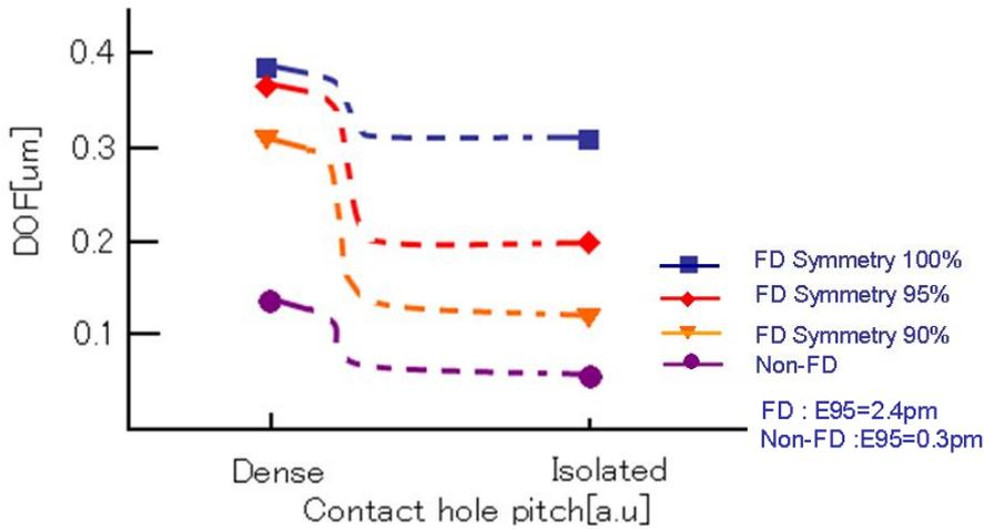
Fig.7: Correlation of contact hole pitch and DOF and its required value.
