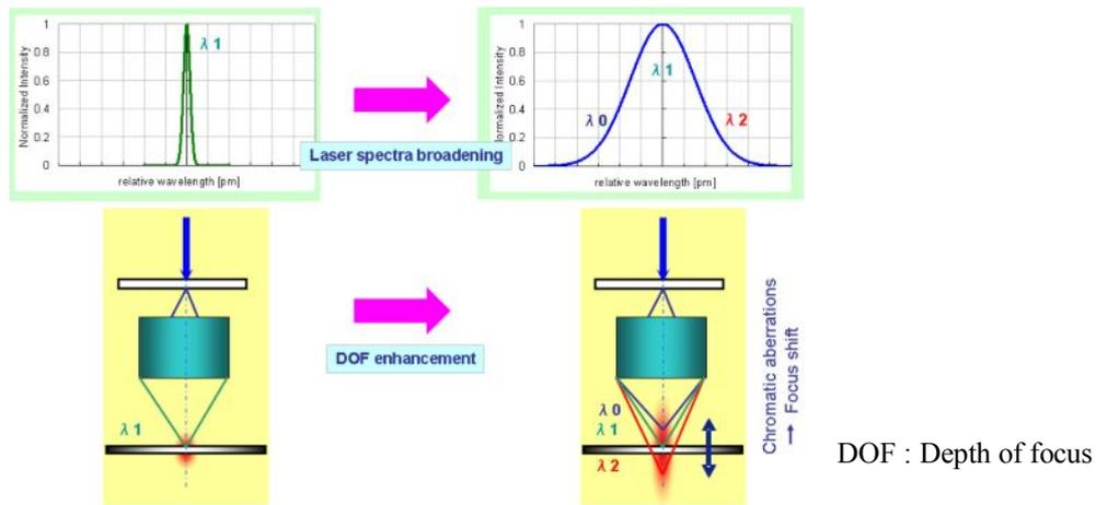
Fig.2: Correlation between spectral bandwidth and focus position
