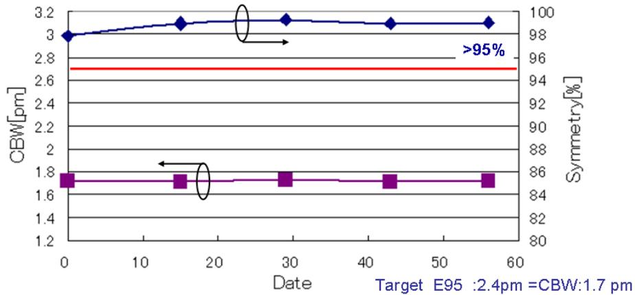
Fig.11: Long term CBW stability and the symmetry of spectral bandwidth
