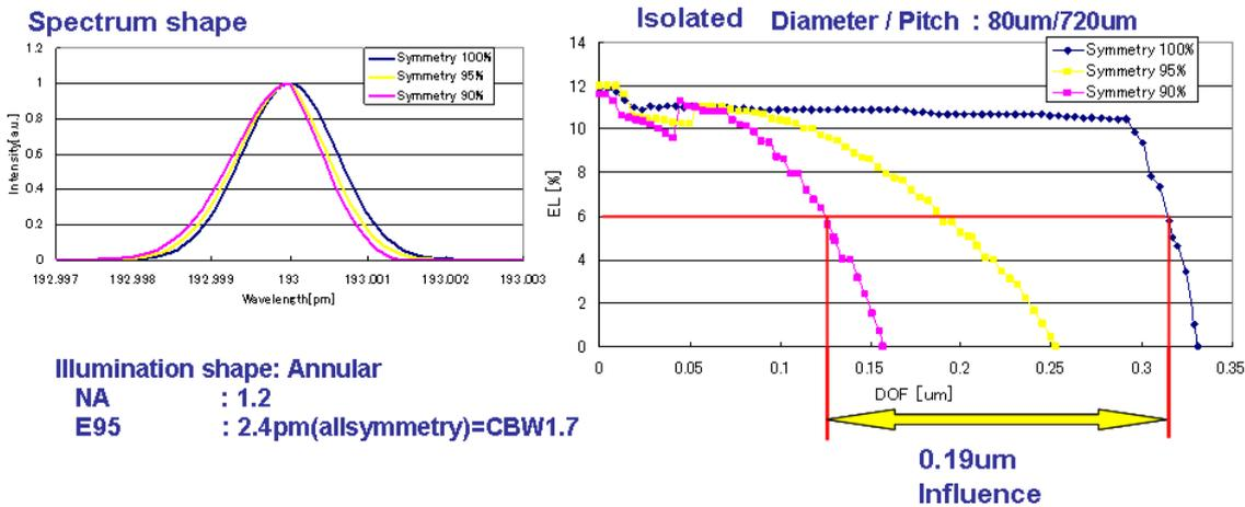
Fig.6: Correlation of the symmetry of spectral shape and DoF (Isolated)
