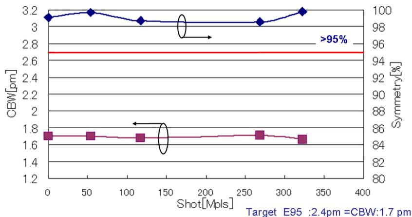
Fig.10: short term CBW stability and the symmetry of the spectral shape
