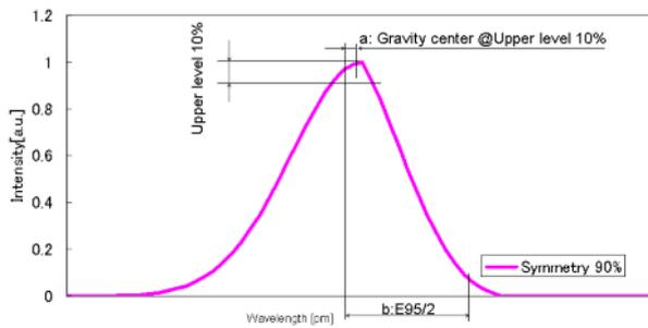
Fig.8: The definition of the symmetry of spectral bandwidth
