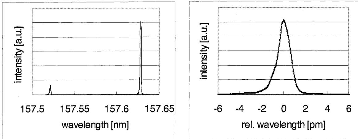
Figure 2: Measured free run F<sub>2</sub> laser spectrum (left) and single-line F<sub>2</sub> spectrum at 157.63nm (right).
