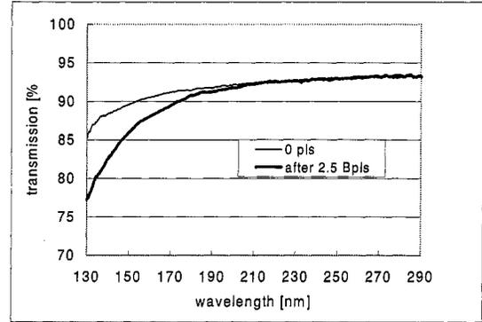
Figure 12: Output coupler transmission before and after 2.5Bpls.
