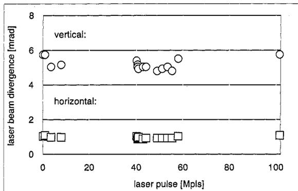
Figure 9: Laser beam divergence at 1/e<sup>2</sup> full width
