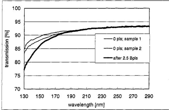
Figure 11: Laser chamber window transmission before and after 2.5Bpls.
