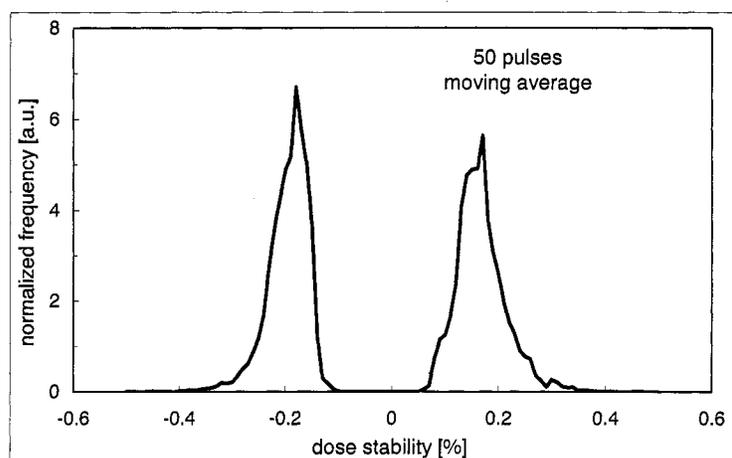
Figure 5: Dose stability (DS) distribution; the plot displays the DS of 50 bursts sampling and 50 pulses moving average during 100Mpls.
