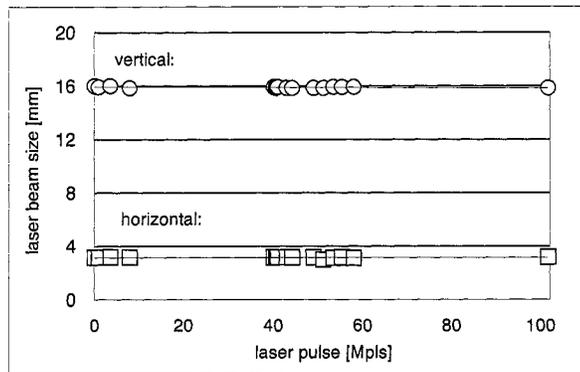
Figure 8: Laser beam size at 1/e<sup>2</sup> full width
