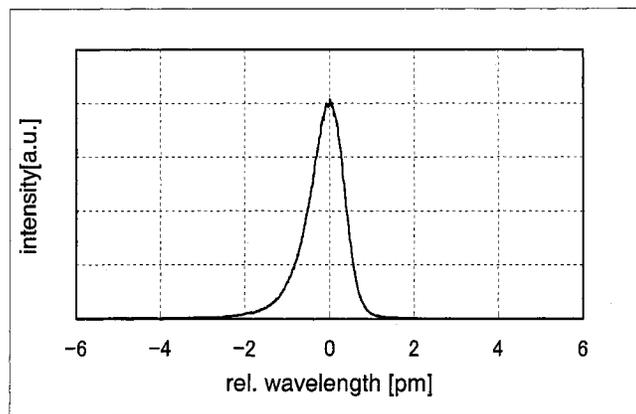
Figure 6: Laser spectral profile; 0.92pm deconvoluted fwhm.
