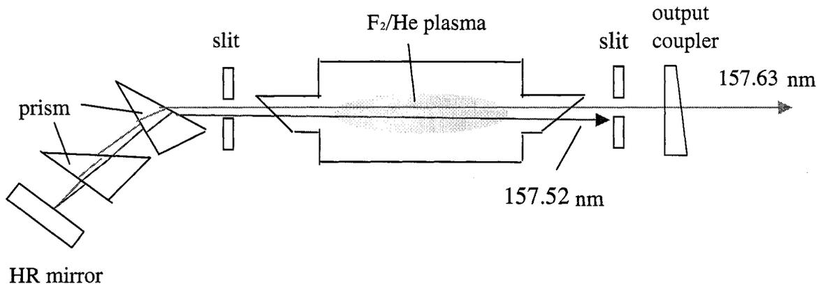
Figure 1: Single line laser resonator.
