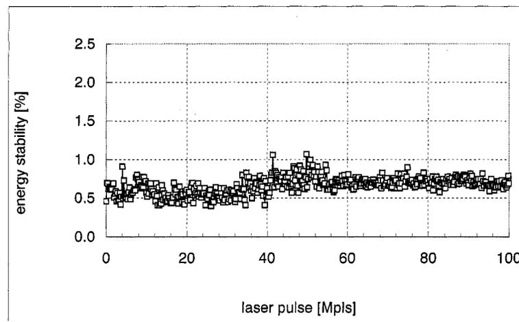
Figure 3: Energy stability; moving average of 50 pulses.
