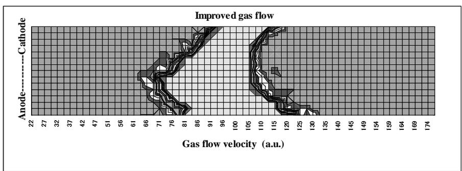
Fig. 1 (b) Gas flow velocity between the cathode and anode – 4kHz KrF
