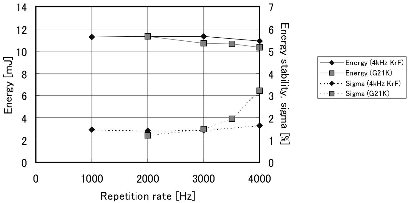
Fig. 4 Frequency characteristics
