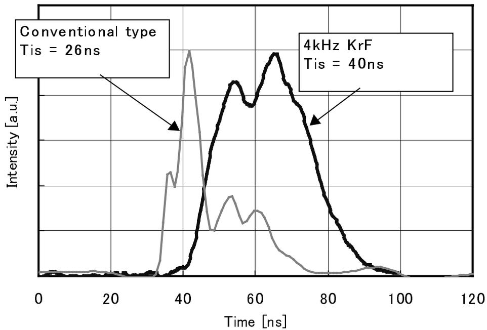
Fig. 7 Output pulse shape
