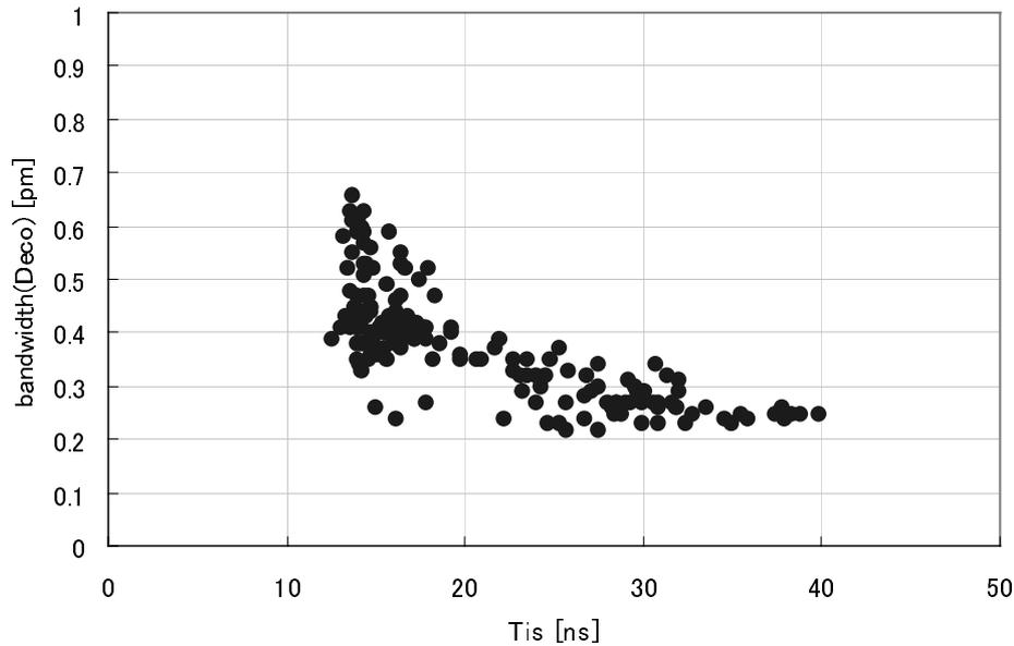
**Fig. 6** Spectrum bandwidth (Deco) versus pulse duration (Tis)
