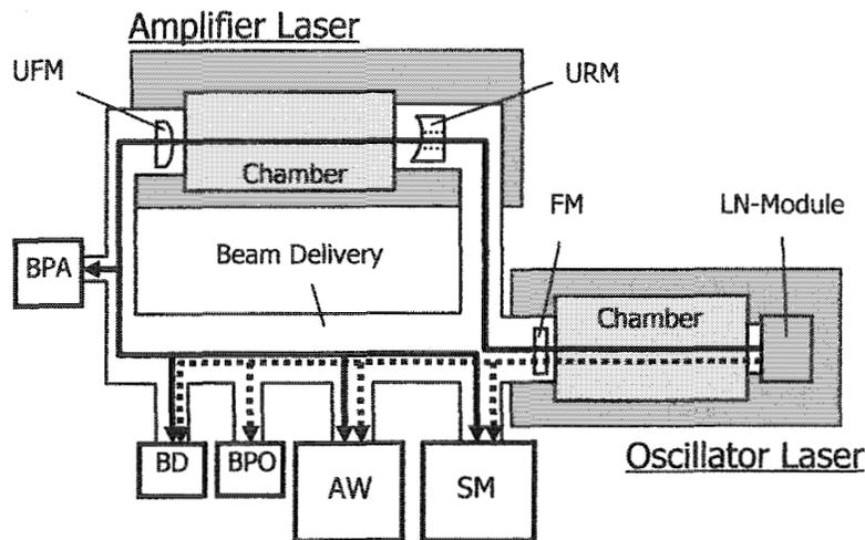
[Fig.2] The 5 kHz Ultra-Line-Narrowed F<sub>2</sub> Laser System
