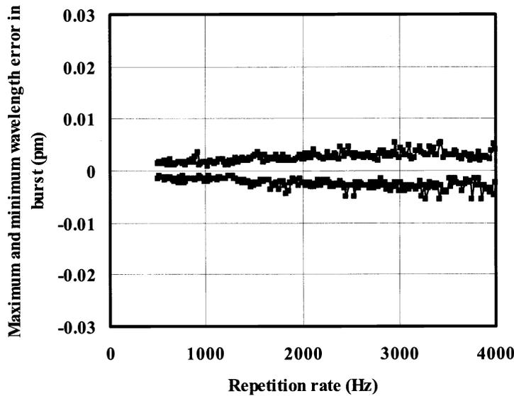
Fig. 5 Average wavelength stability dependency on repetition rate (50 pulse window)
