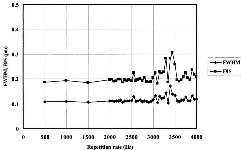
Fig. 4 Spectrum dependency on repetition rate.
