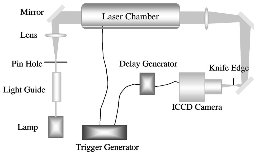
Fig. 3. Schlieren measurement system
