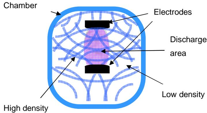
Fig. 1 Image of acoustic wave behavior in a laser chamber
