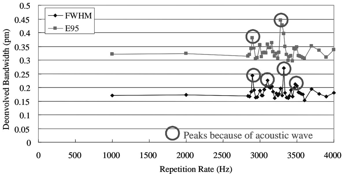
Fig. 2. Effect of acoustic wave on spectra bandwidth (non-ideal chamber)
