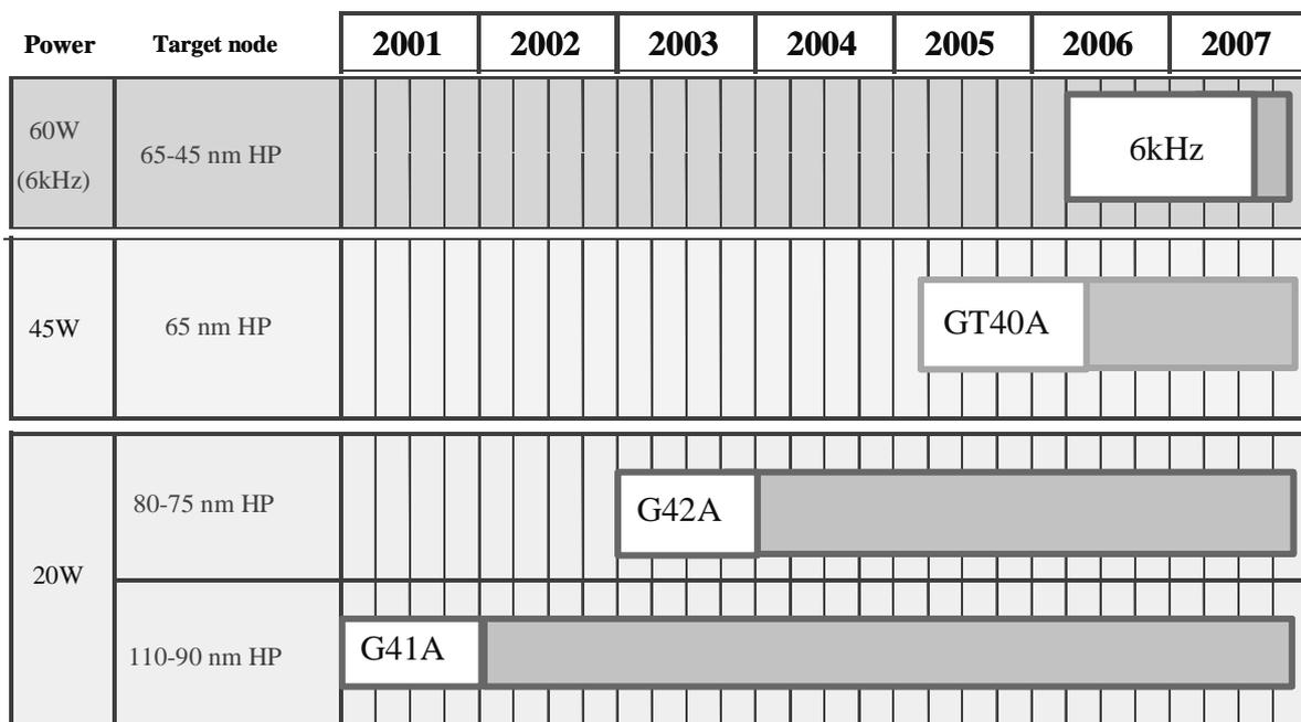
Fig. 9. Gigaphoton roadmap for ArF excimer laser.
