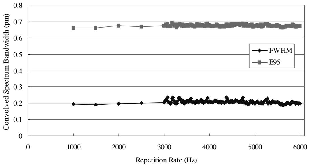
Fig. 8. Spectral bandwidths of improved laser chamber from 1 kHz to 6 kHz operation
