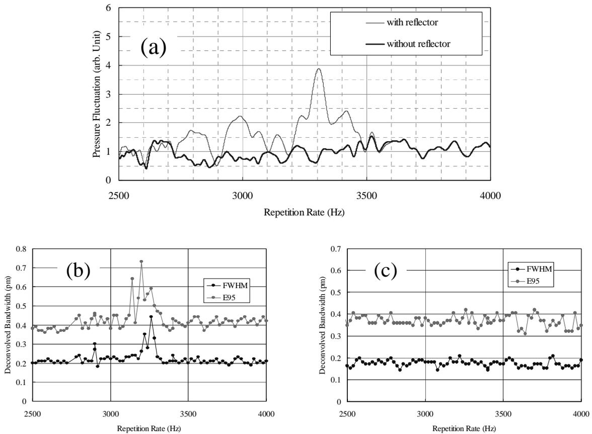
Figs 6. (a) Gas fluctuation calculation results and spectral bandwidths measurements (b) with reflector and (c) without reflector
