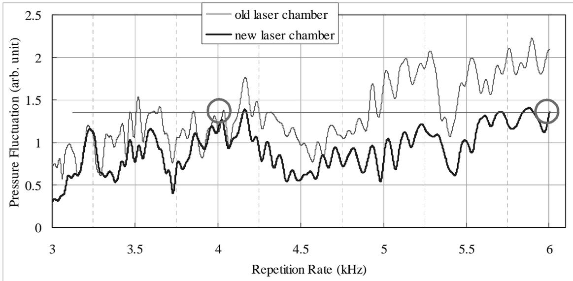
Fig. 7. Calculation results for new laser chamber
