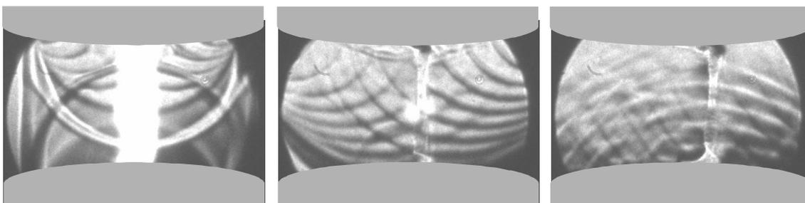
Figs 4. Visualized acoustic wave (measured by Schlieren method)
