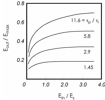
Figure.2 Calculated power extraction vs. pulse energy relations plotted for different values of the  $\tau_p/\tau_r$  parameter ( $\tau_p = 1$  ns,  $P(20)$ )<sup>16)</sup>.
