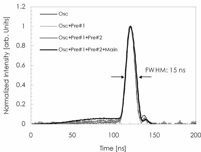
Figure.4 Input pulse of the EO Q-switched  $CO_2$  oscillator and amplified laser pulses after each stage
