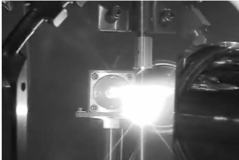
Figure.7 Xenon plasma by 1 kW (repetition rate: 100 kHz, pulse width in FWHM: 15 ns) CO<sub>2</sub> laser irradiation
