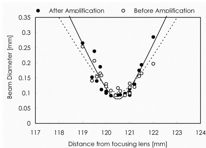
Figure.6 Dependence of focused beam diameter on the distance from the focusing lens
