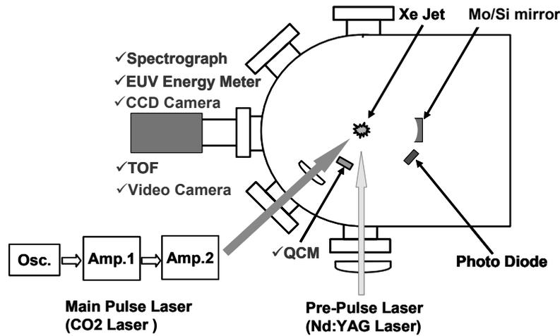
Fig. 1 Experimental setup for the pre-pulsed CO<sub>2</sub> laser plasma characterization
