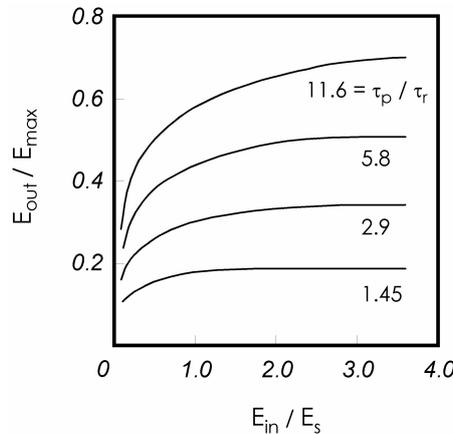
Figure.14 Calculated power extraction vs. pulse energy relations plotted for different values of the  $\tau_p/\tau_r$  parameter ( $\tau_p = 1$  ns, P(20))<sup>8</sup>.
