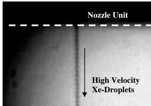
Fig.9. High velocity Xe droplets in high vacuum
