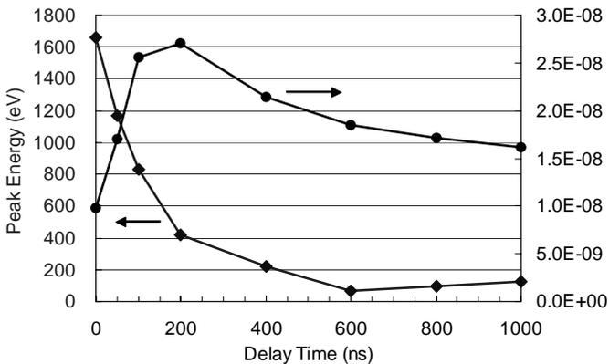
Fig.10. Peak ion energy distribution dependence on delay time
