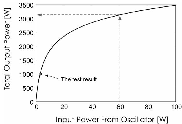
Figure.15 Output power estimation of the RF-excited MOPA system by use of a short pulse 60 W input power from an oscillator. The amplification test result with 1 kW output is plotted.
