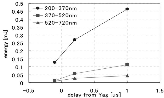
Fig.4 Out-of-band energy distribution dependence on delay time
