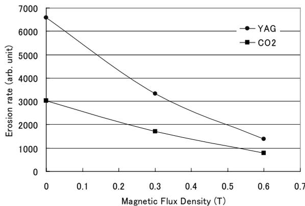
Fig.11. Erosion rate dependence on magnetic flux density
