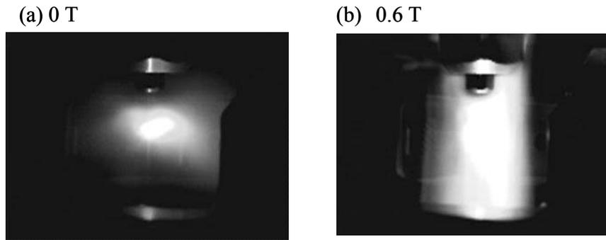
Fig.12. CO<sub>2</sub> laser produced plasma source image in a visible range (a) without and (b) with 0.6-T magnetic field.
