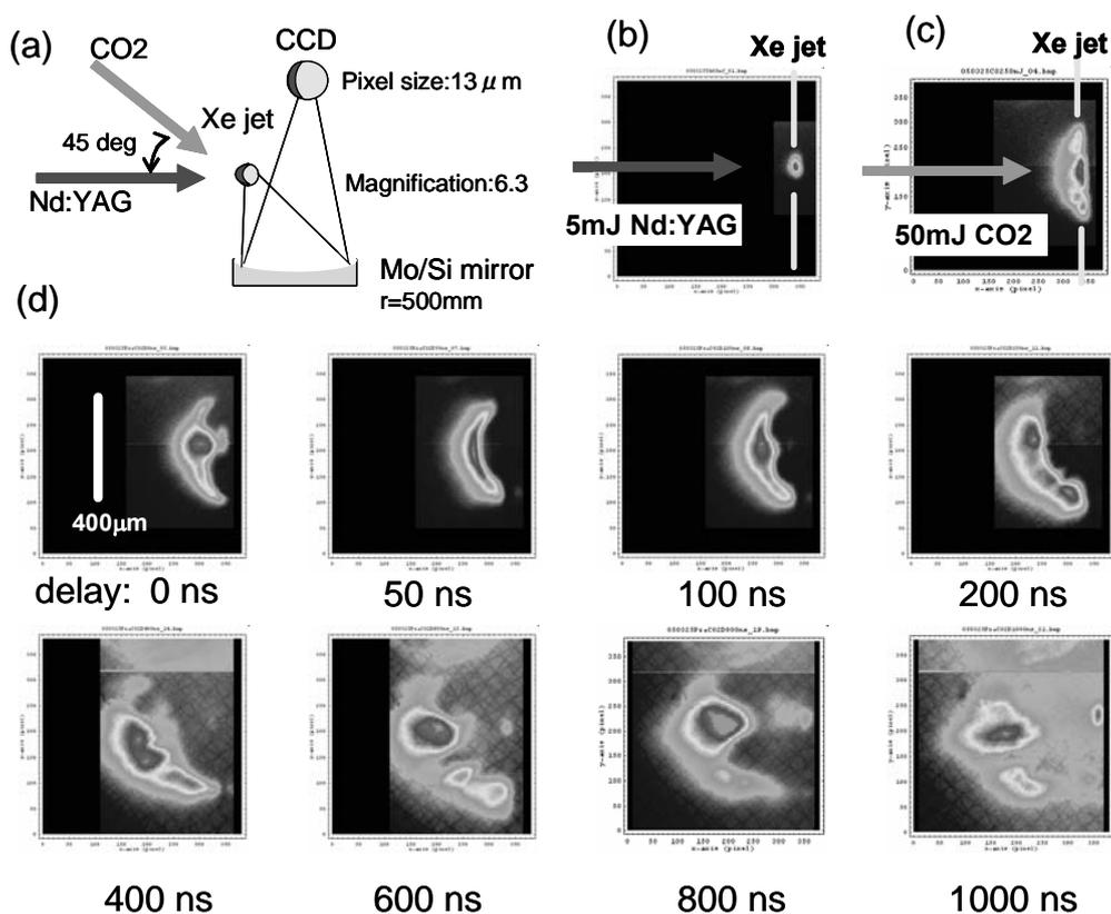
Fig.3. EUV plasma image monitored by a Mo/Si multilayer concaved mirror and a CCD camera.
