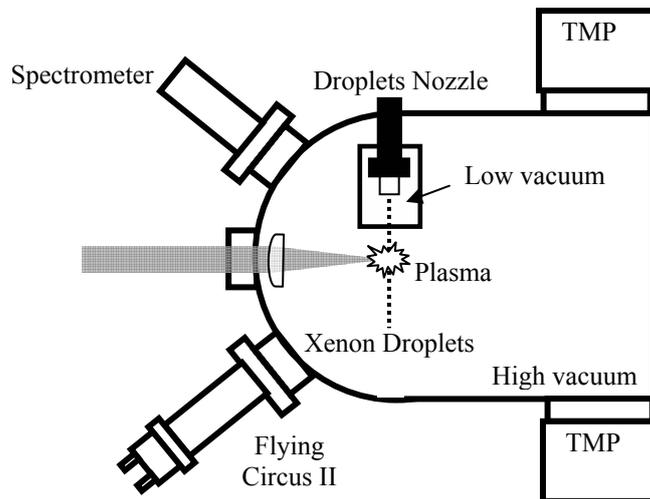
Fig.5. Schematic of the droplet generation and laser irradiation system
