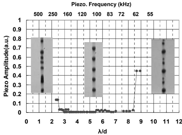
Fig.6 Relationship between piezo amplitude and  $\lambda/d$  for uniform droplets generation
