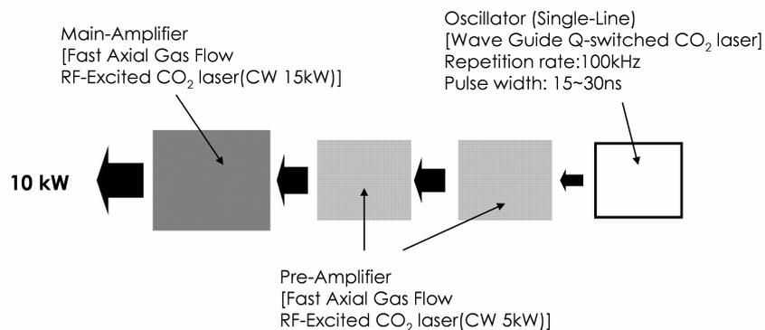
Figure.13 Configuration of the laser driver based on RF-pumped fast axial flow CO<sub>2</sub> laser
