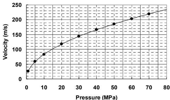
Fig.8 Xenon droplets velocity vs. pressure
