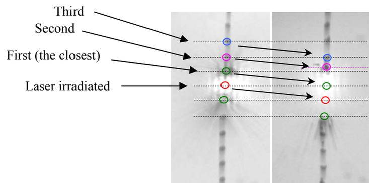
Fig.7 Droplets behavior under laser irradiation (Left: 0 delay, Right: 10  $\mu$  sec delay)
