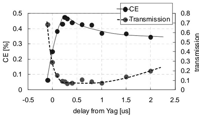
Fig. 2 CE and the CO<sub>2</sub> laser transmittance dependence on the delay time
