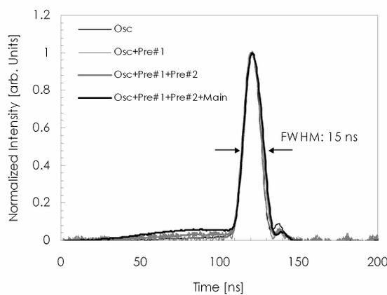
Figure.16 Input pulse shape of the EO Q-switched CO<sub>2</sub> oscillator and amplified laser pulseshapes after each stage
