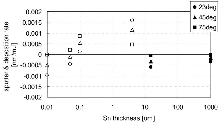
Fig.11. QCM results of various Sn targets as a function of the Sn thickness.
