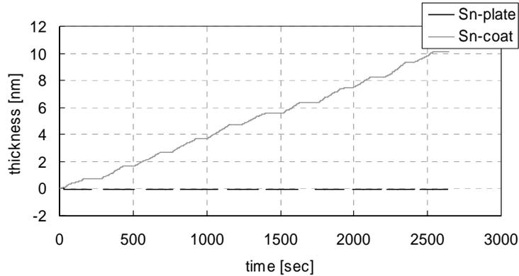
Fig.12. QCM result for a Sn-plate and a 800nm Sn coated glass substrate.
