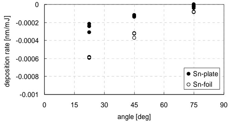
Fig. 6. The QCM results of the solid Sn-plate and Sn-foil target for different measurement angles with CO<sub>2</sub> laser.
