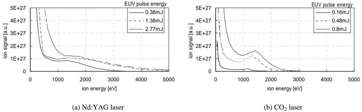
Fig. 8. Ion waveforms generated by the Nd:YAG and CO<sub>2</sub> laser.
