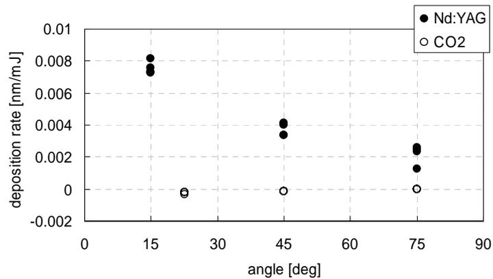
Fig. 7. Solid Sn-plate QCM results for Nd:YAG and CO<sub>2</sub> drive laser.
