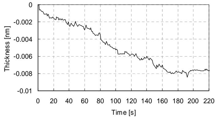
Fig. 5. A typical QCM signal for the Sn-plate target with CO<sub>2</sub> laser.
