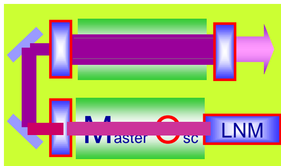
Fig.2 A schematic of the injection lock (MOPO)system
