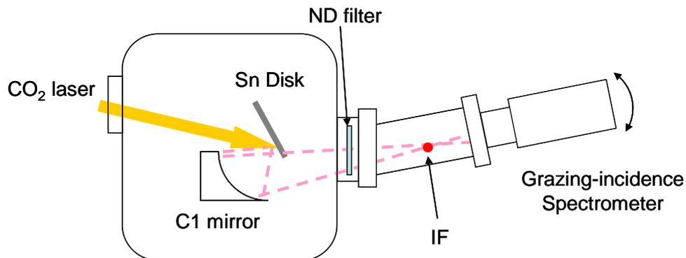
Fig.9 EUV spectrum measurement configuration at intermediate focus
