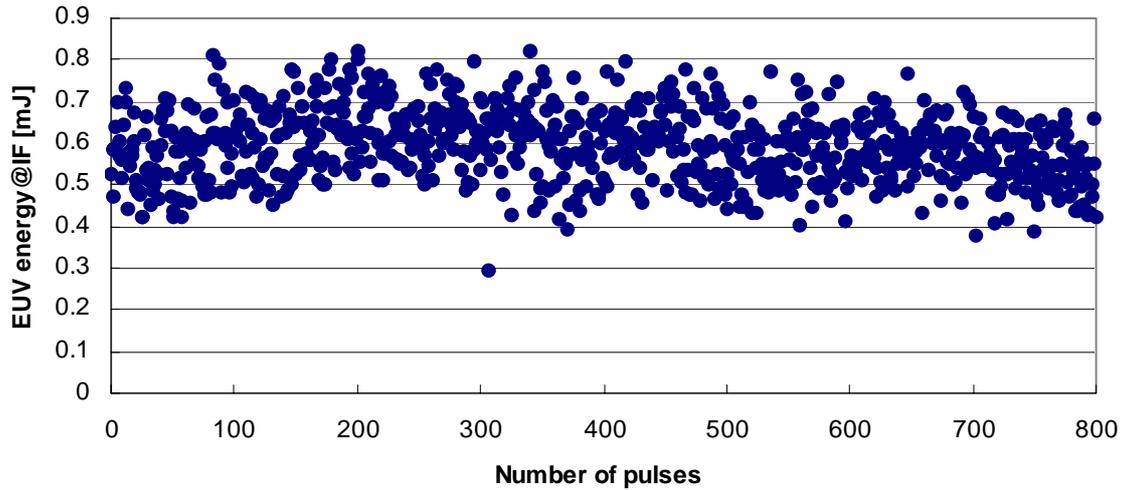
Fig. 5. EUV pulse energy stability at intermediate focus.
