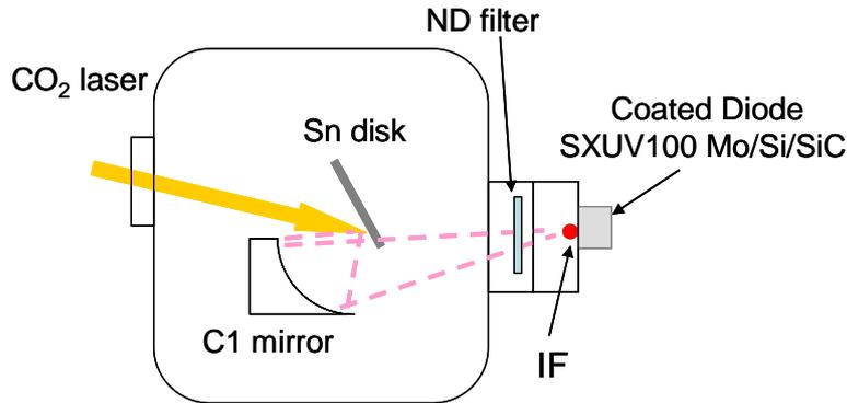
Fig.3 EUV energy measurement configuration at intermediate focus
