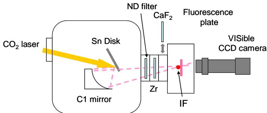
Fig.7 EUV profile measurement configuration at intermediate focus
