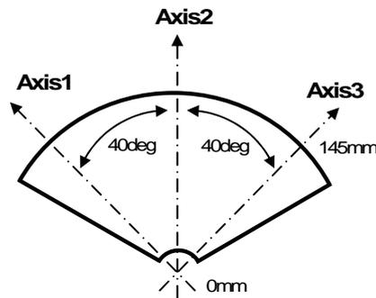
a) mirror geometry and axis directions of mirror measurements
