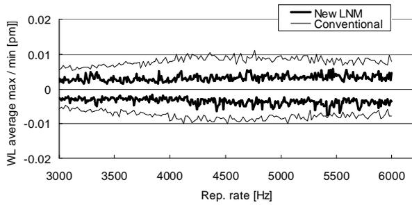
Figure 4. The repetition rate dependency of wavelength error
