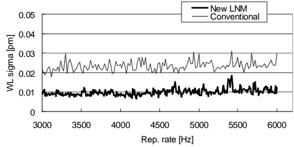
Figure 5. The repetition rate dependency of wavelength sigma
