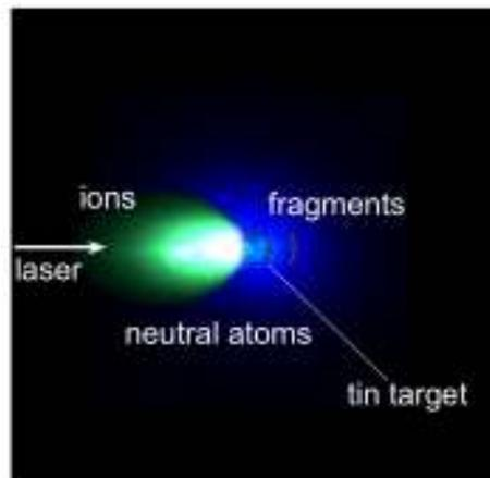
Figure 11 Components coming from pre-pulse irradiated droplet (image)
