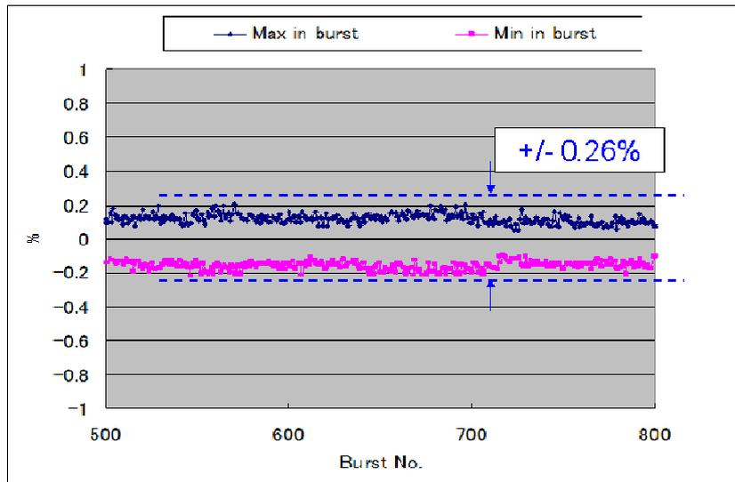
Figure 13-2 EUV dose data (closed loop simulation)
