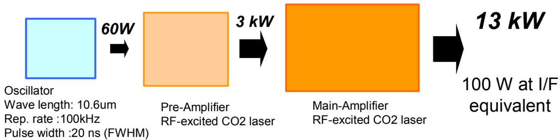
Figure 6 Configuration of the CO<sub>2</sub> MOPA system.
