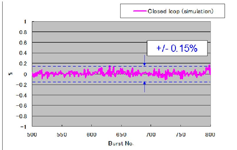
Figure 13-1 EUV stability data (closed loop simulation)
