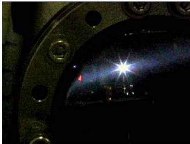
Figure 9 Picture of magnetic field guided LPP plasma
