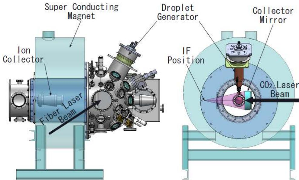
Figure 2 EUV chamber of ETS device
