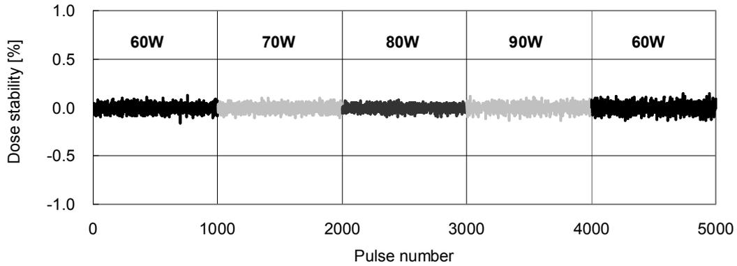
Figure 2. Dose stability from 60 to 90W
