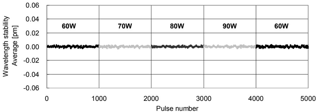
Figure 3. Wavelength stability error from 60 to 90W
