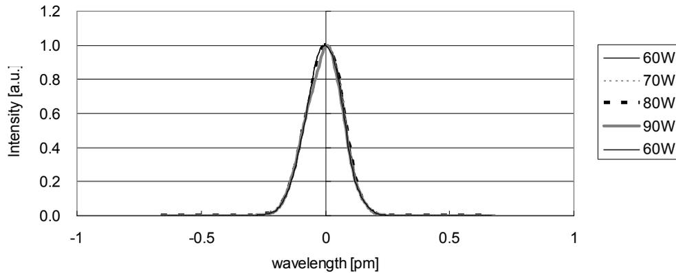
Figure 6. Spectral profile shape from 60 to 90W
