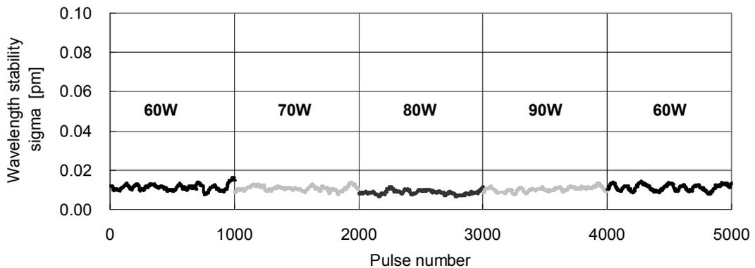
Figure 4. Wavelength stability sigma from 60 to 90W
