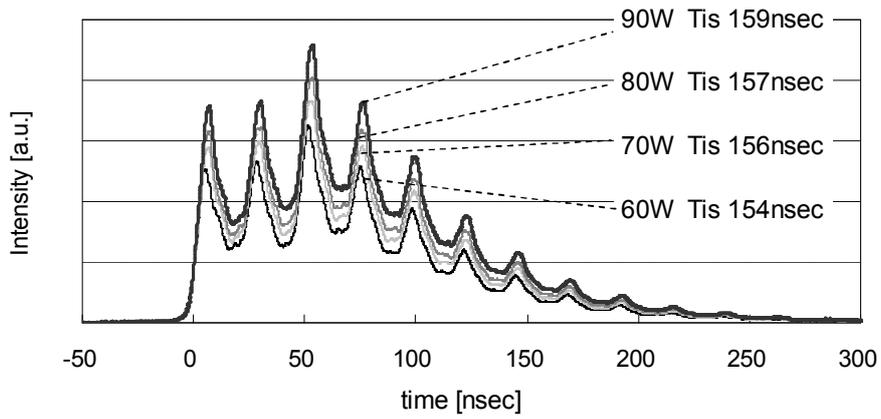
Figure 7. Laser pulse shape and the pulse duration
