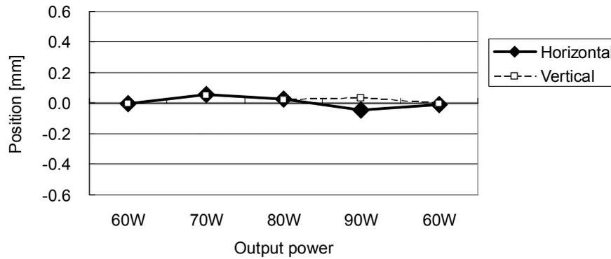
Figure 10. Output power dependency of beam position
