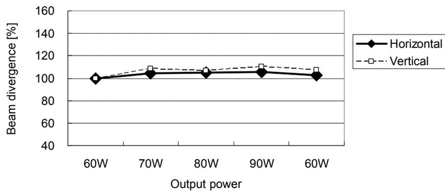
Figure 9. Output power dependency of beam divergence
