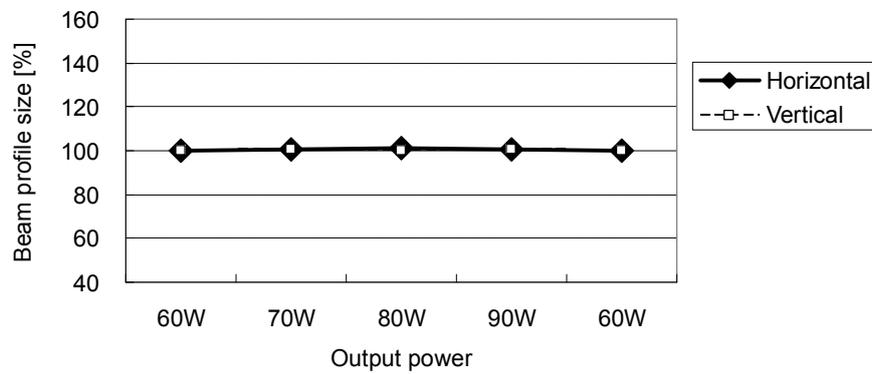
Figure 8. Output power dependency of beam profile size
