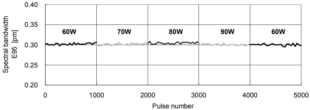
Figure 5. Spectral bandwidth from 60 to 90W
