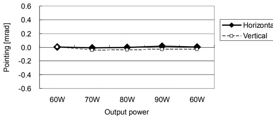
Figure 11. Output power dependency of beam pointing
