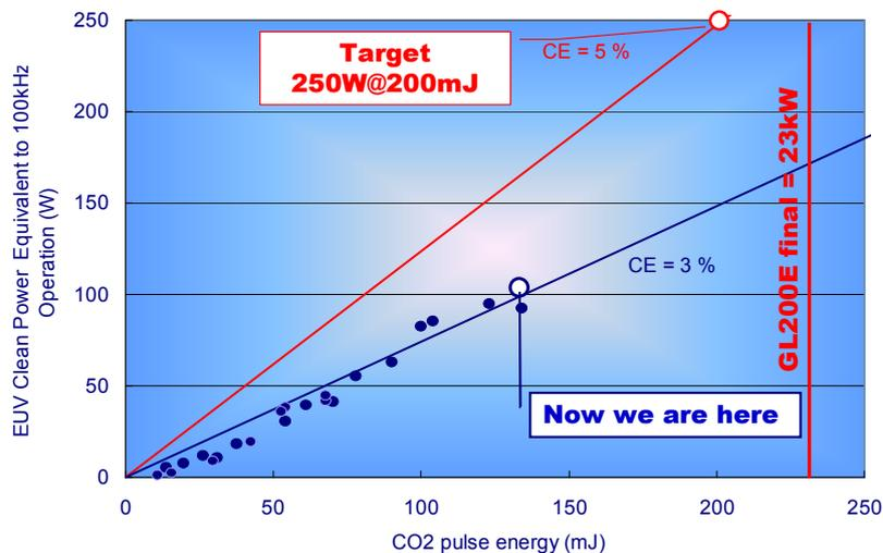
Figure 13 Scalability of CO2 energy and EUV power
