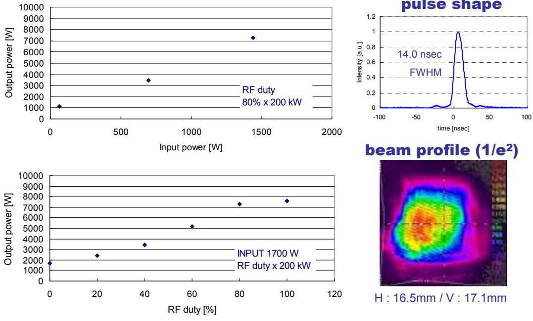
Figure 10 Beam profile of CO<sub>2</sub> laser
