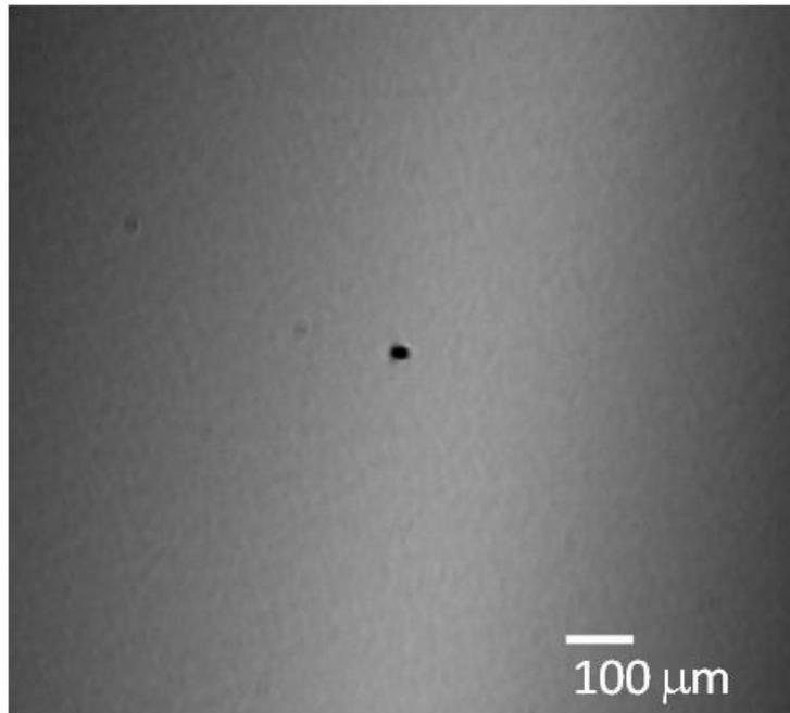
Figure 5. Shadowgraph image of 20 μm diameter Sn droplet
