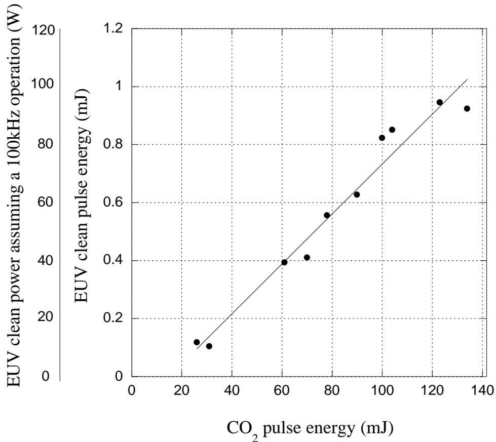
Figure 11. CO<sub>2</sub> pulse energy vs., EUV clean pulse energy
