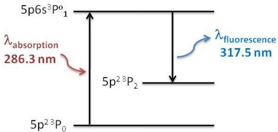
Figure 6. Energy level of Sn atom
