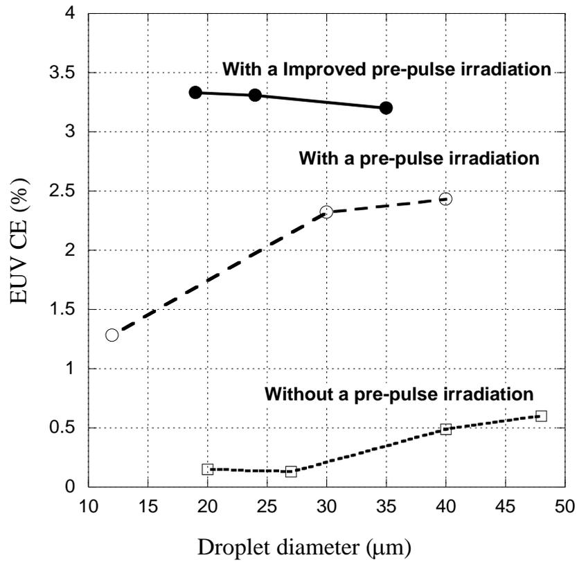
Figure 10. EUV CE as a function of the droplet diameter
