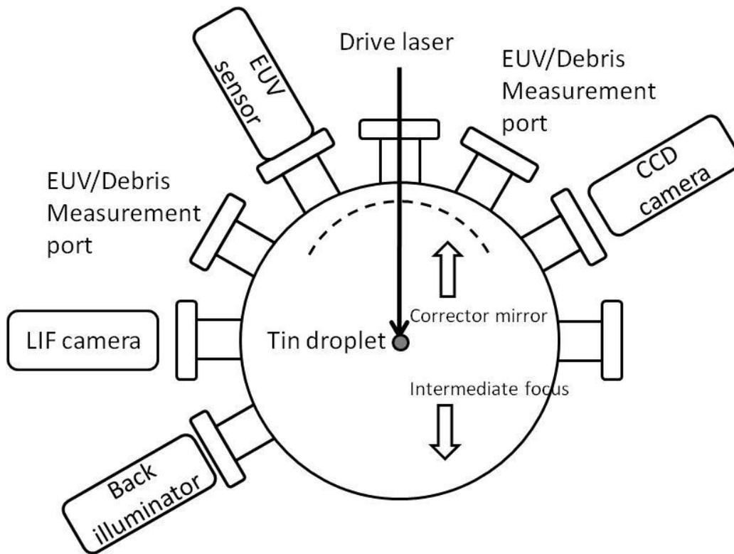
Figure 3. Experimental setup for basic investigation of EUV light generation and tin particles mitigation
