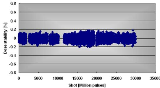
Fig.3 Dose stability trend in the durability test
