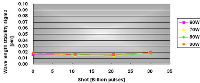
Fig.6 . Wavelength stability error from 60 to 90W
