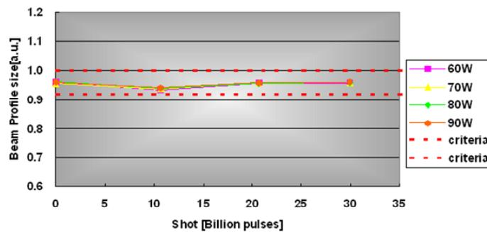
Fig.7 Output power dependency of beam profile size
