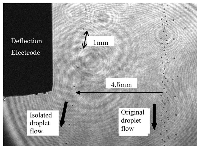
Fig. 8. Isolated Sn droplets
