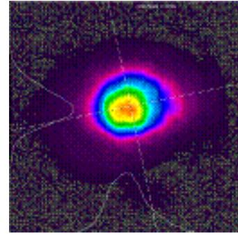
Fig4. Typical profile of the output laser beam.
