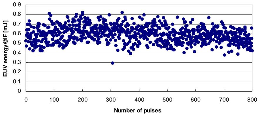
Fig. 5. EUV pulse energy stability at an IF point.
