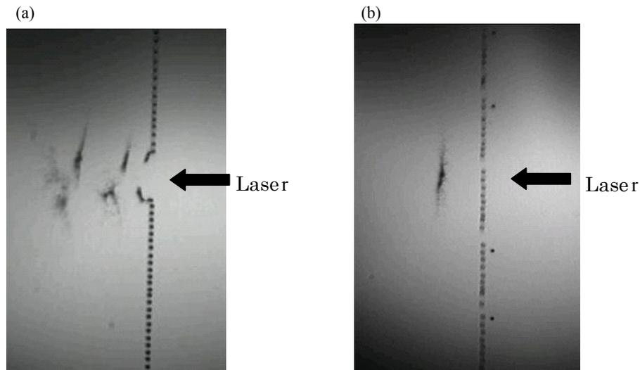
Fig. 9. Images taken 4 $\mu\text{s}$  after laser irradiation onto a) continuous droplets b) isolated droplet.
