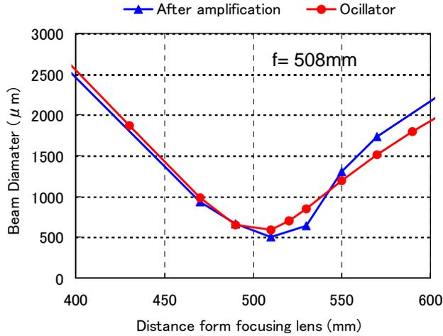
Fig. 3. Focus ability of the CO<sub>2</sub> laser beam.
