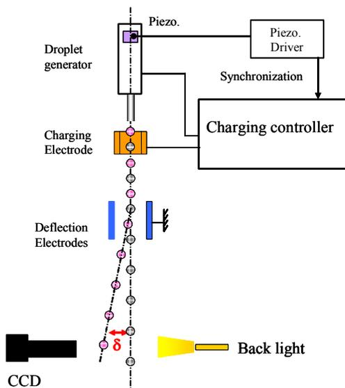
Fig. 7. Schematic of droplet generator and selection system.
