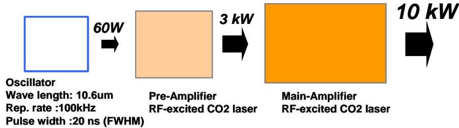
Fig.1. Configuration of the CO<sub>2</sub> MOPA system.
