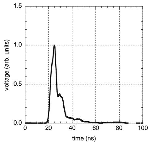
**Fig. 6** Temporal profile of the drive laser pulse.
