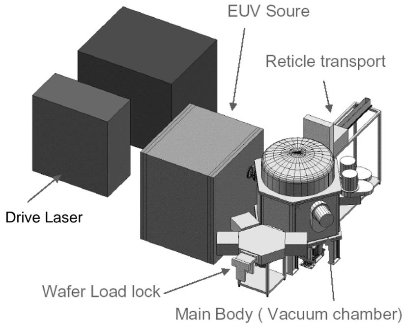
**Fig. 1** Schematic of SFET.
