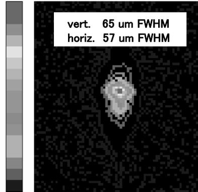
**Fig. 5** Laser spot size at Xe jet position.
