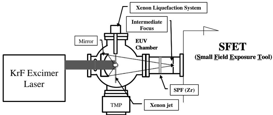
**Fig. 2** Schematic of the light source.
